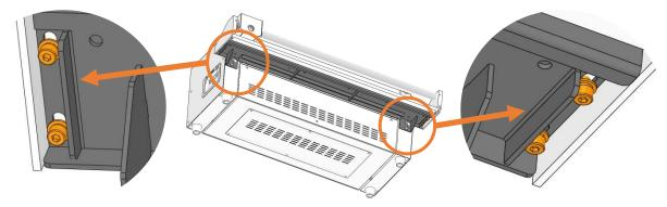
Step2:Move the cutter towards the machine and test the paper cutting effect.
