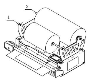
When the machine is first powered on or the alarm has been recovered, if the machine needs to be fed after determining that the roll is without paper, you can do the following: 1. The MG tissue paper is into the support rod-1, die-cut kraft paper roll is into the support rod -2
