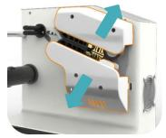
a. Loosen the 4 screws located on the upper and lower covers with a 3mm wrench and remove the upper and lower covers (2 on the upper cover and 2 on the lower cover).
