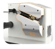
a. Use a 3mm Allen wrench to install the upper and lower cover with the 4 screws.
